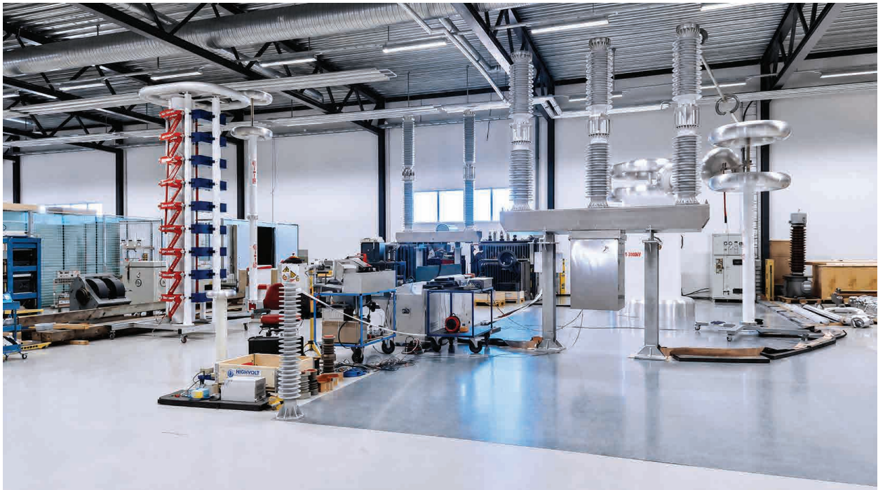
Testing of solid insulated vacuum circuit breaker in the inhouse high voltage test laboratory,
