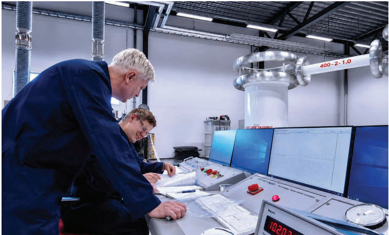
Inhouse high voltage test laboratory, 400kV power frequency and PD test, 900kV 60kJ impulse test system
