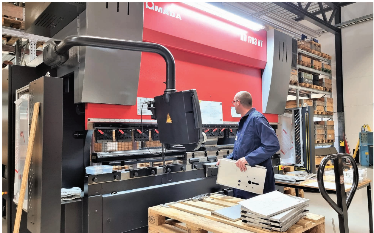
8 axes 170t automatic press brake for processing sheet metal parts
