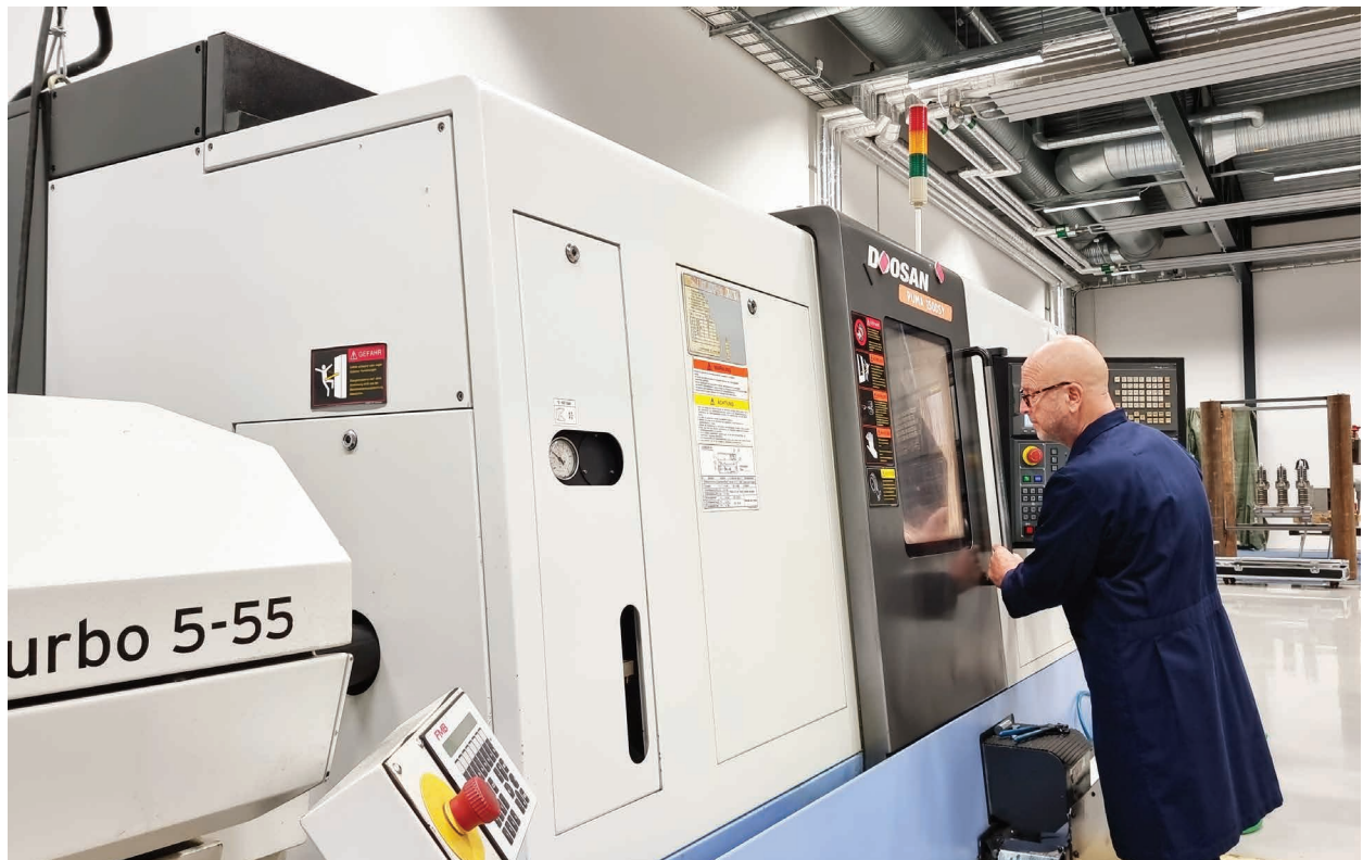
Multi spindle lathe with automatic magazine
