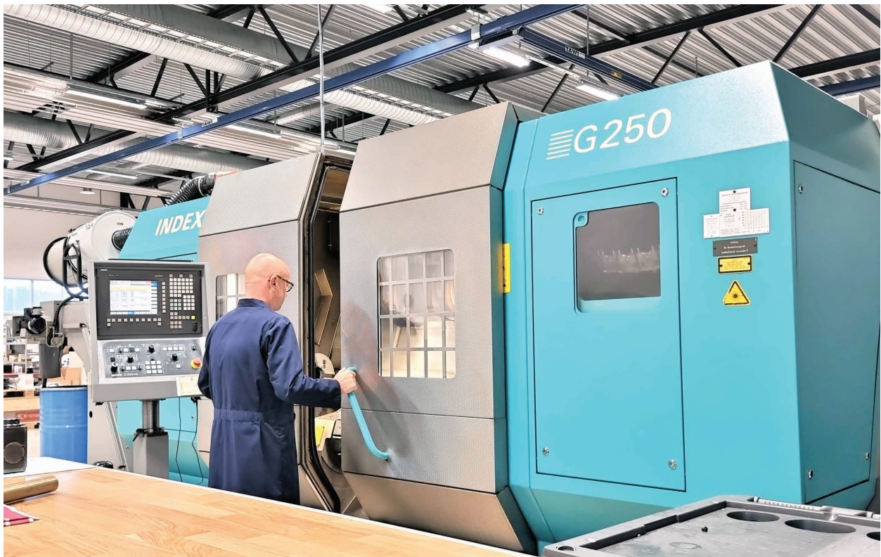
Multi spindle lathe with 5 axes milling capabilities
