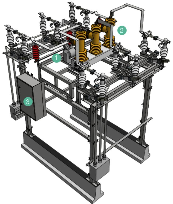
Installation of the TVS450 set inside of a sectionalizing scheme.
